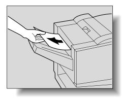
**8** Open the transport guide, and then pull out any misfed paper in the transport section.
